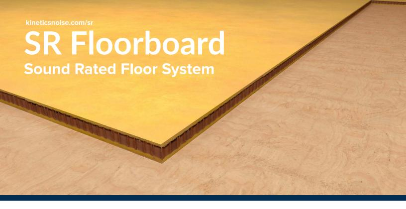
Kinetics SR Floorboard is a unique sound underlayment material which substantially reduces sound transmission through hard surface floor systems. SR Floorboard offers better airborne noise control than Soundmatt, while being thinner than the Ultra Quiet SR. This underlayment arrives at the jobsite as 4' x 8' x 5/8" sheets of high density molded glass fibers separated by a rigid honeycomb core.
