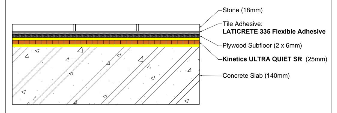
Important Note: An IIC rating will generally be 5 points higher than a F-IIC (AIIC) rating. The IIC is conducted at a laboratory where flanking is controlled. The F-IIC (AIIC) is conducted in the field where flanking is not as controllable, hence the 5 point difference.
